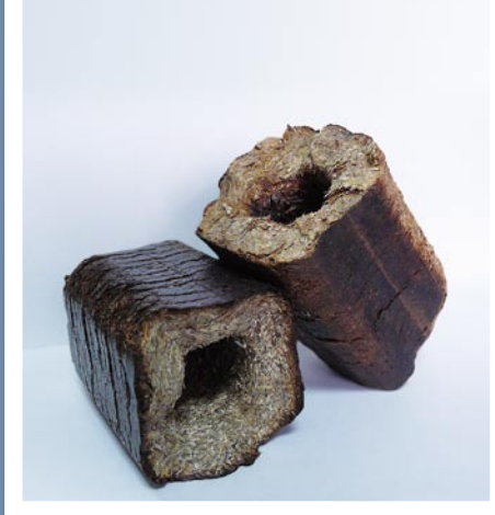
Trial fuel briquettes produced from biomass harvested in Sporava mire, Belarus photo Uladzimir Malashevich
